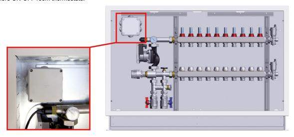
The wiring case has all the connections required for the regulation unit: boiler enable signal (NO), room thermostat (TA), safety thermostat (TS) and pump power (POMPA). It has to be powered at 230V.
