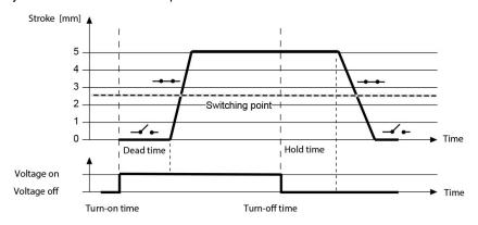
The valve is opened steadily by the plunger motion upon switching on the operating voltage and after expiry of the Dead time. After the operating voltage is cut and after expiry of the Hold time the valve is closed evenly by the closing force of the compression spring. The actuating force of the compression spring is matched to the actuating force of commercially available valves and keeps the NO valves closed when de-energized.
