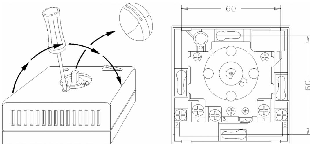
In order to don't damage the switch is recommended to remove the cover following the direction indicated by the arrow.
