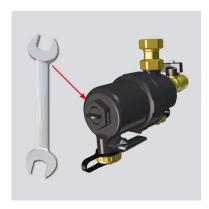
To inspect the desludger completely or clean/replace the filter cartridge, you can remove the cup completely with a normal CH 29 wrench. Lubricate the o-rings with EPDM compatible grease.
